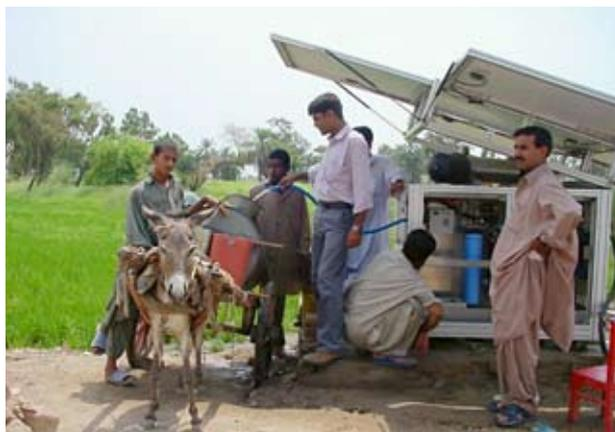
The Trunz Water Systems cleans 900 liters per hour and draws its energy from solar panels or windmills.
